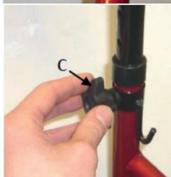
Attach the plastic washer and tightening handle 'C' onto the screw. Rotate the tightening handle clockwise until it secures the handlebar into position.
